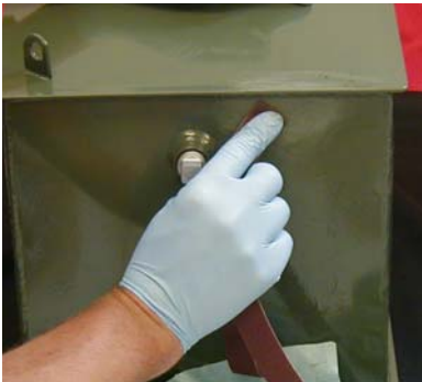
Sand or brush repair area
